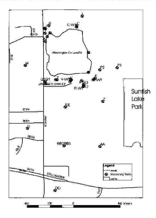
Figure 2 Ground Water Monitoring Network around Washington County Landfill
