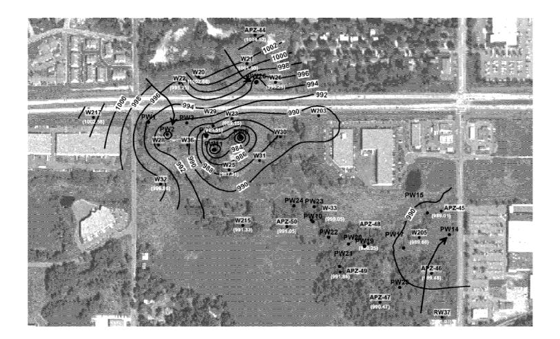
Groundwater Elevation Contour Map Lower Alluvium Aquifer 24 January 2013 - 1st Quarter
